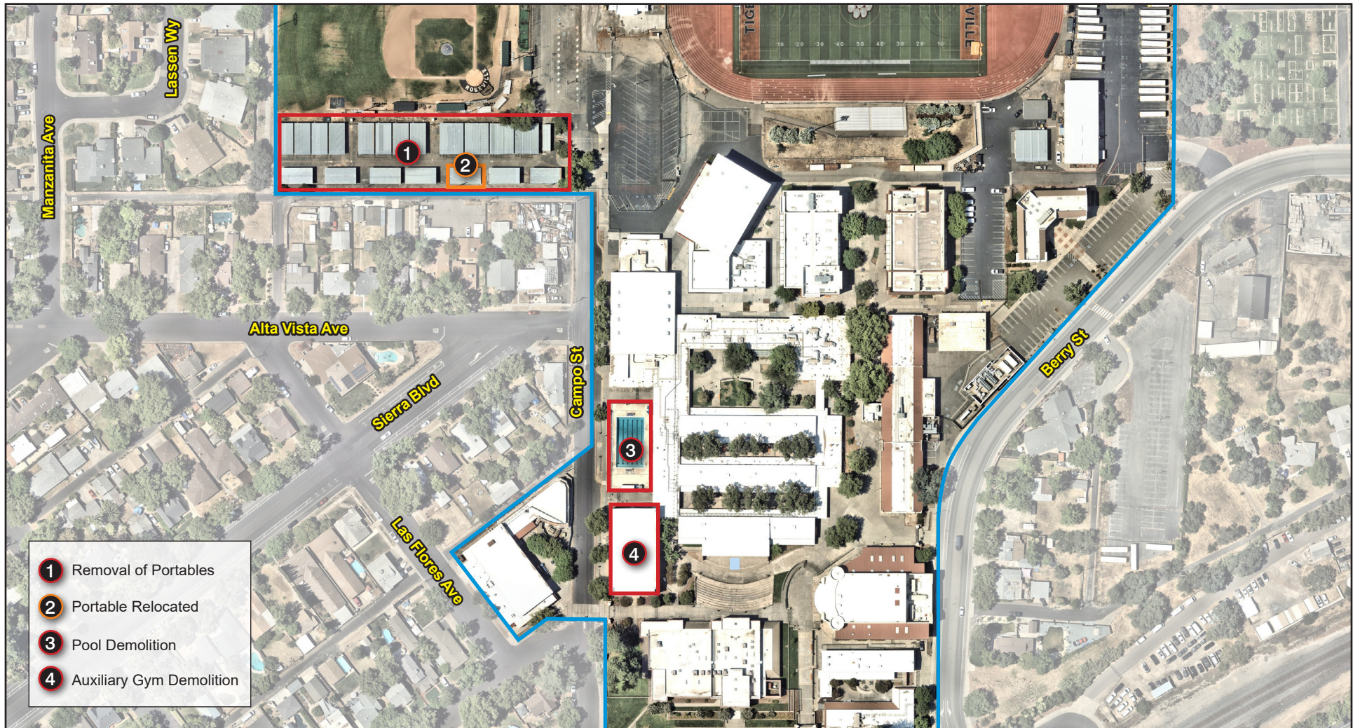
Figure 5 - Demolition and Removal of Portables
