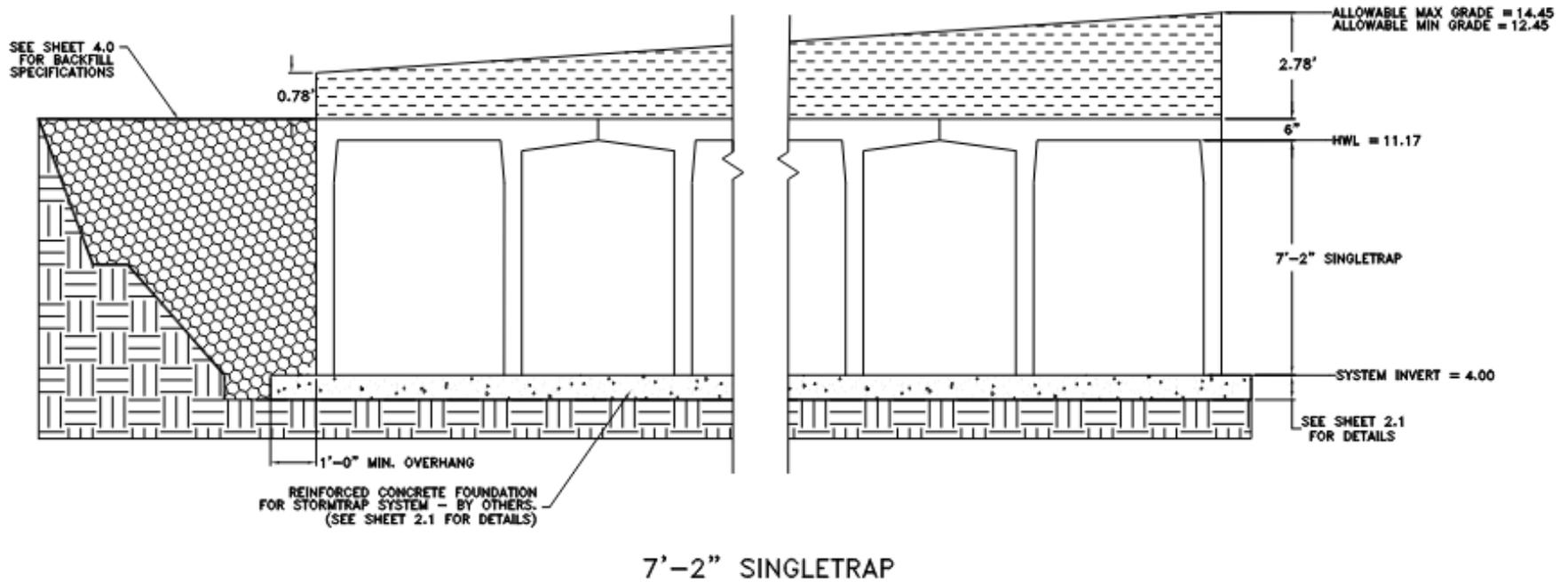
**Basin 100 (BMP 1) – Underground Storage Facility (StormTrap) – Section Detail**
