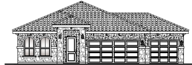
Upgraded Elevation 'B' w/ OPTIONAL 3RD CAR GARAGE, LOFT PLATE & STONE VENEER
