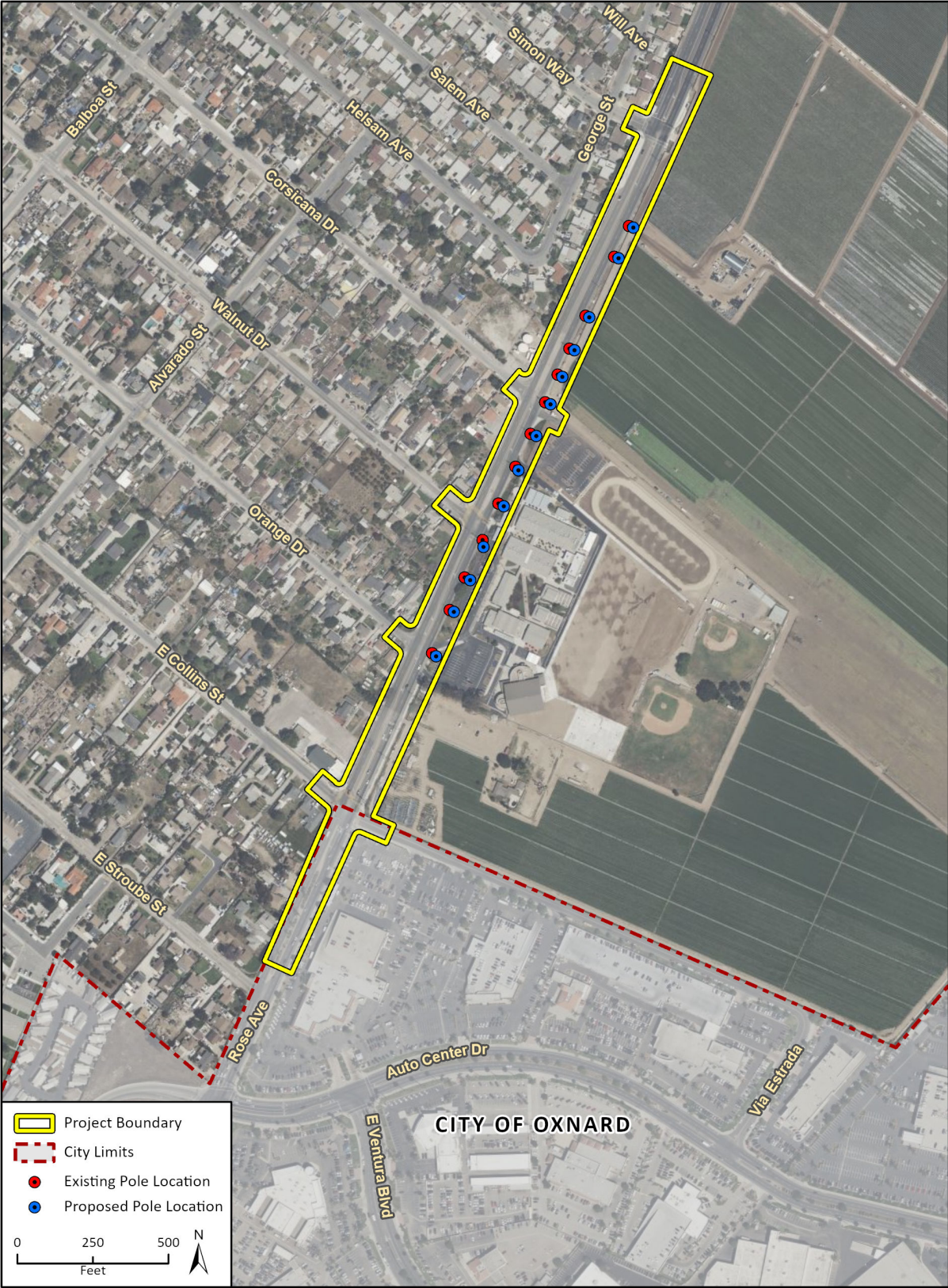
Figure 5 Proposed Utility Pole Relocations – Southern Segment
