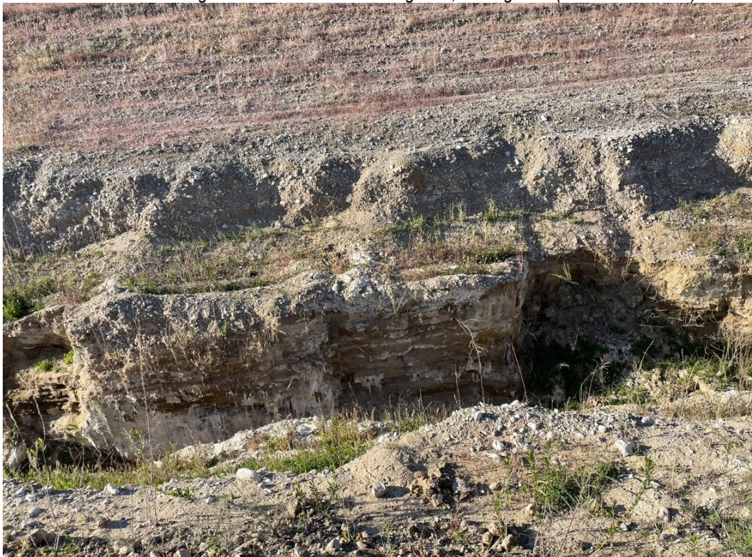
Photo 2: Historical exploratory test pit along northern toe of slope within the Triangle Pit that was used to determine the depth to the Corcoran Clay, looking North (taken 03-07-2022)
