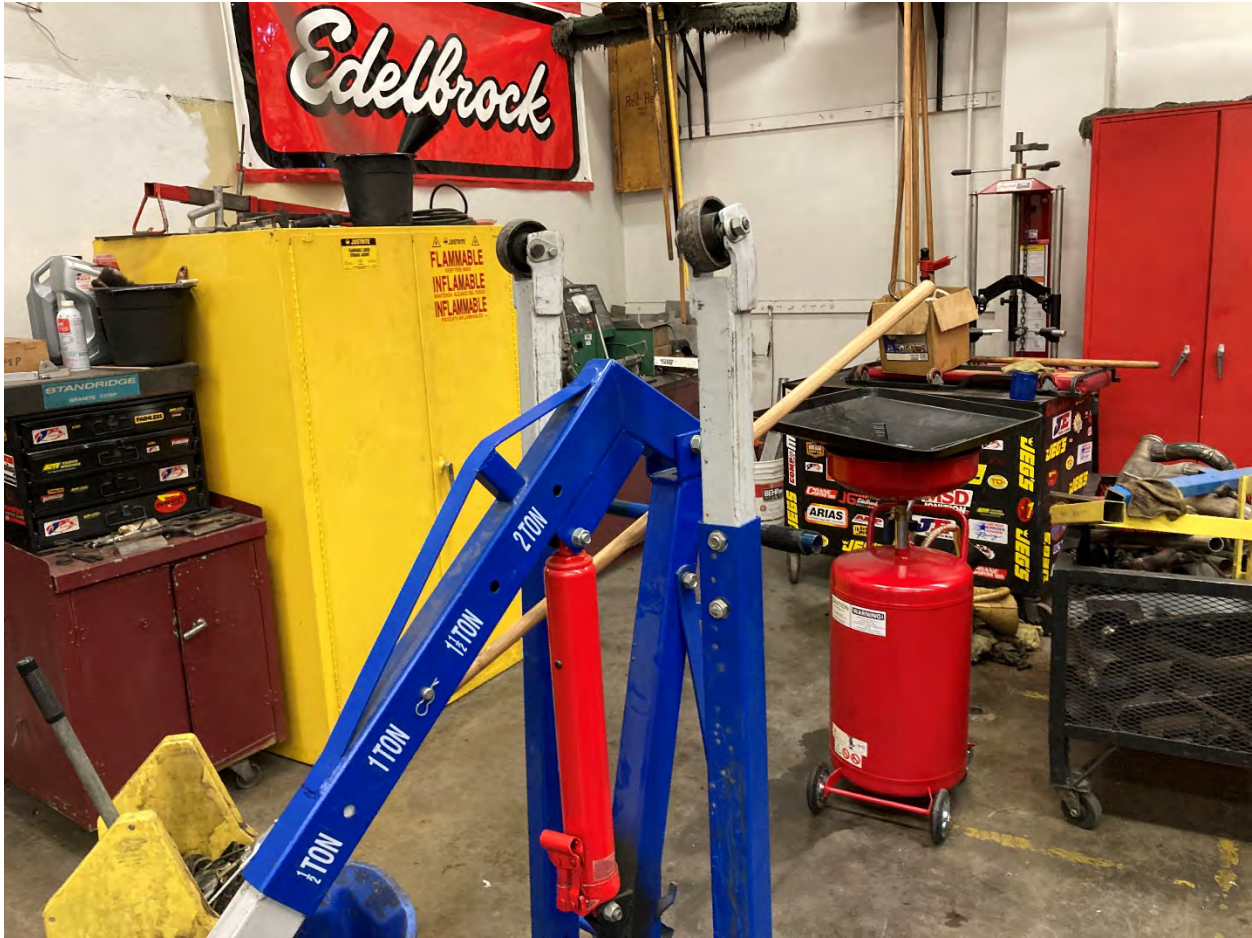
Auto shop interior north wall. Hydraulic lifts and hoists observed along with pneumatic tools and equipment. Flammable storage box observed.
