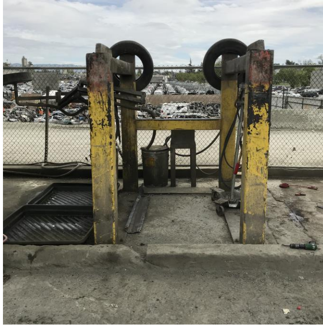
Photograph 15: Gasoline-draining location on Pick-N-Pull portion of the Site.
