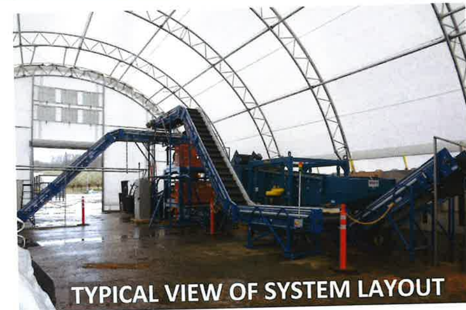
PROCESSED WOOD DRYER SYSTEM FOR FEED MATERIAL INTO GASIFIER UNITS.
