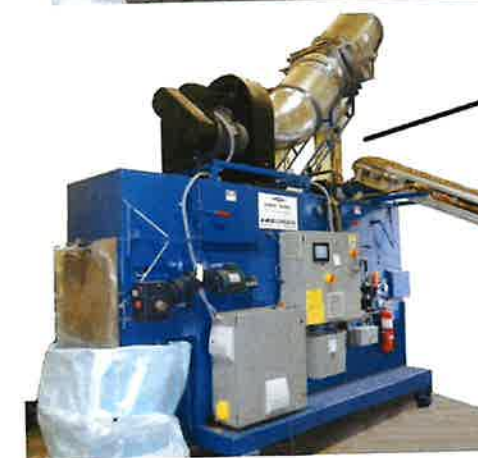
PROCESSED WOOD DRYER SYSTEM FOR FEED MATERIAL INTO GASIFIER UNITS.
