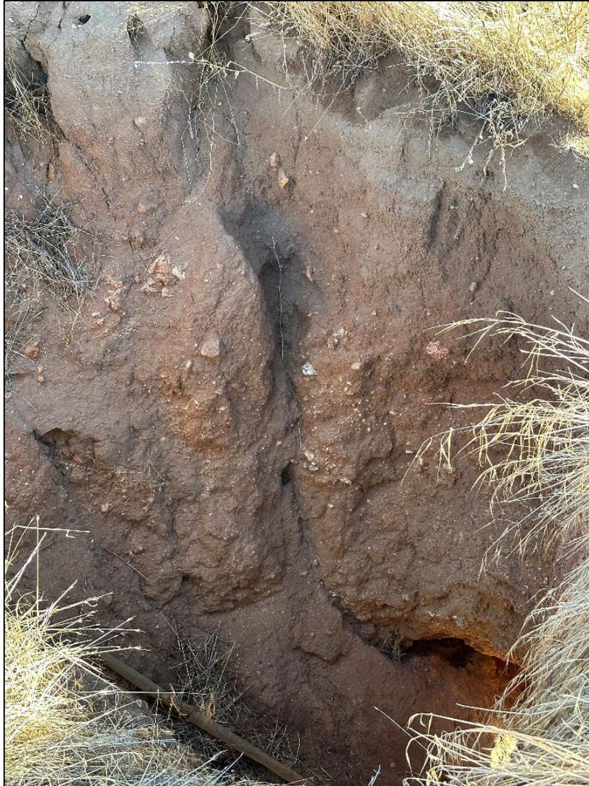
**Figure 6-3** Detailed view of an approximately 8-foot-thick section of the southwest bank of Montgomery Creek at the east-central border of the Project area showing deposits of Qw.
