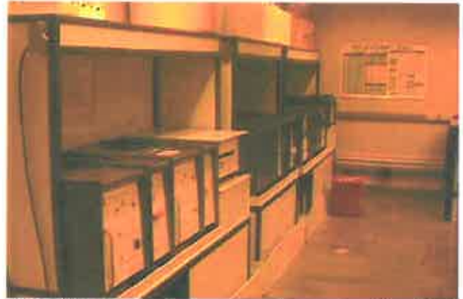
Photo #8: Kepro system in PCB Etch Room for making circuit board prototypes — second set of tanks in background are old system for putting copper onto circuit boards (no longer used)
