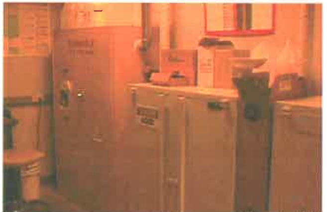
Photo #16: Hazardous materials storage cabinets in PCB Etch Room
