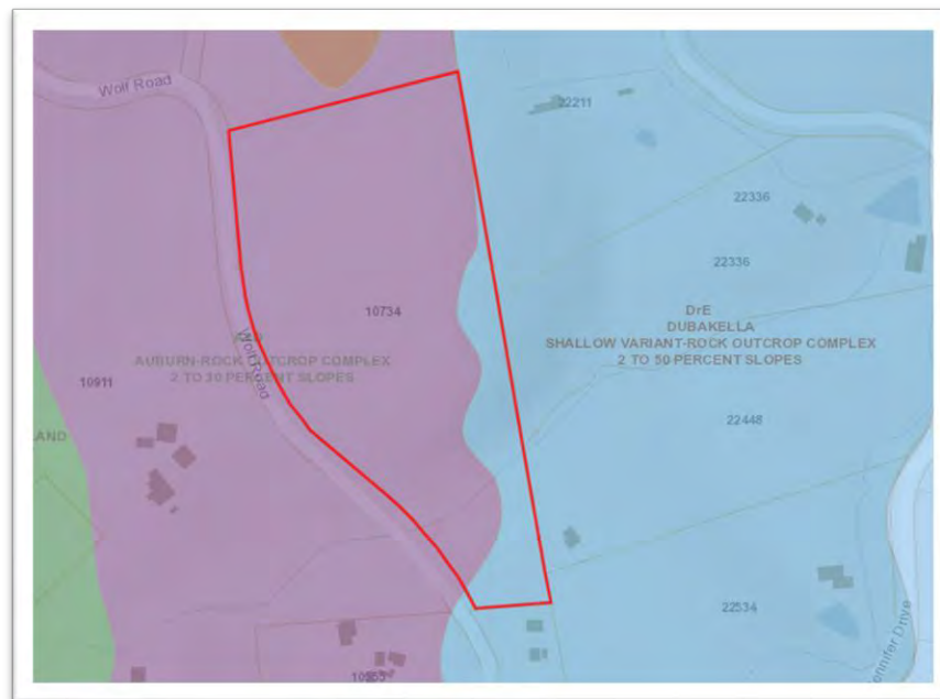
Figure 6 - Soil Types at Project Site
