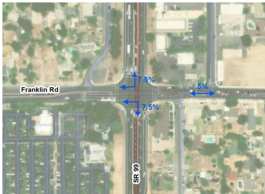
Figure 11. Primary Project Trip Distribution at SR 99 & Franklin Rd
