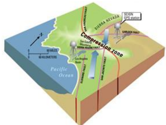
A schematic block model of Southern California showing the motion of the Pacific and North American plates, and the big bend of the San Andreas fault where the plates squeeze together.
