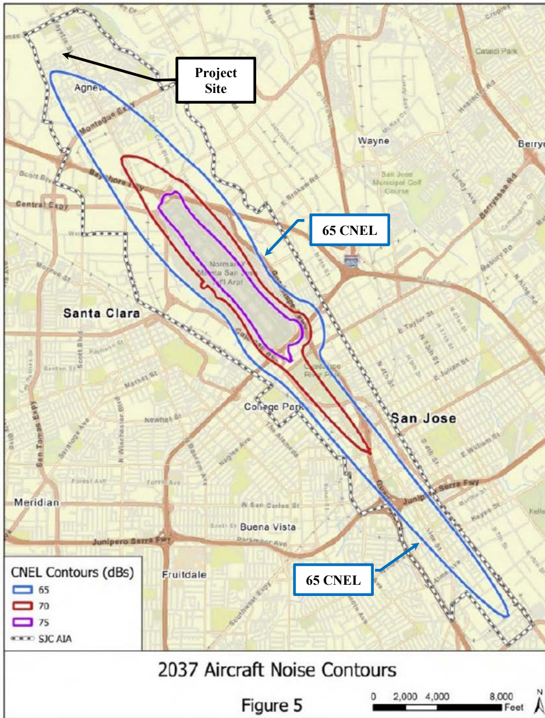
FIGURE 3 2037 CNEL Noise Contours for ALUC Plan in Santa Clara County Relative to Project Site
