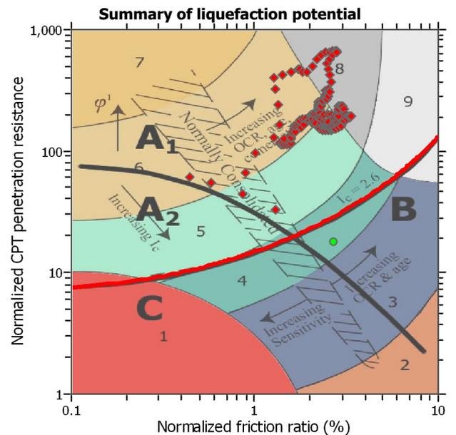
Zone A<sub>1</sub>: Cyclic liquefaction likely depending on size and duration of cyclic loading
