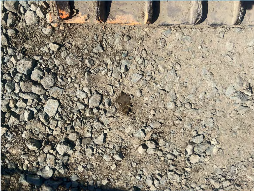
Photograph 5: Representative soil composition of imported gravel and artificial fill across the project site. September 13, 2023
