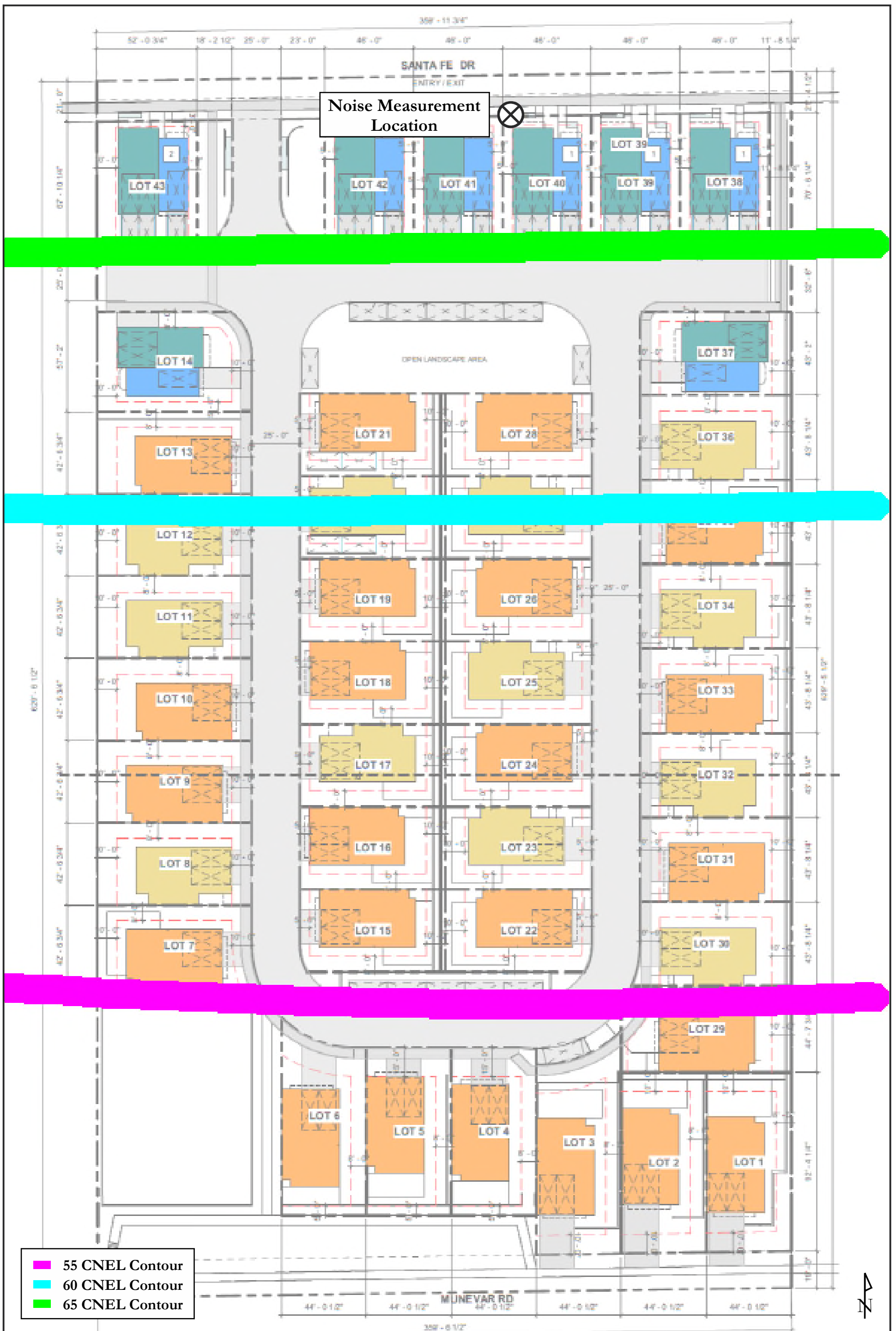
Site Plan Showing Current Traffic CNEL Noise Contours and Noise Measurement Location Job # S200805.3
