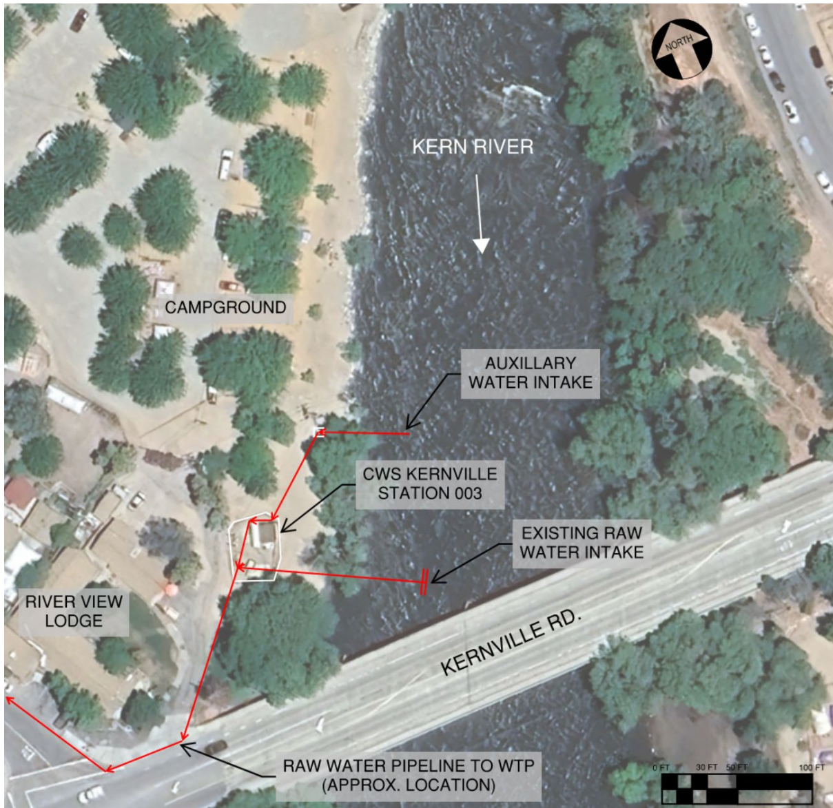
Figure 3 Existing Raw Water Intake System Location
