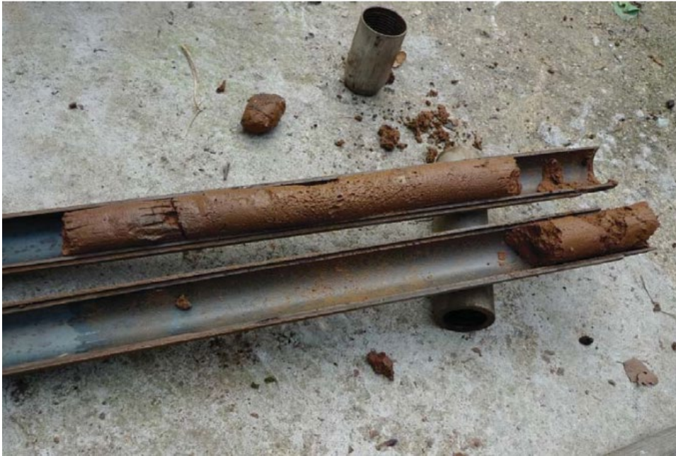
Standard Penetration Test (SPT) Sample
