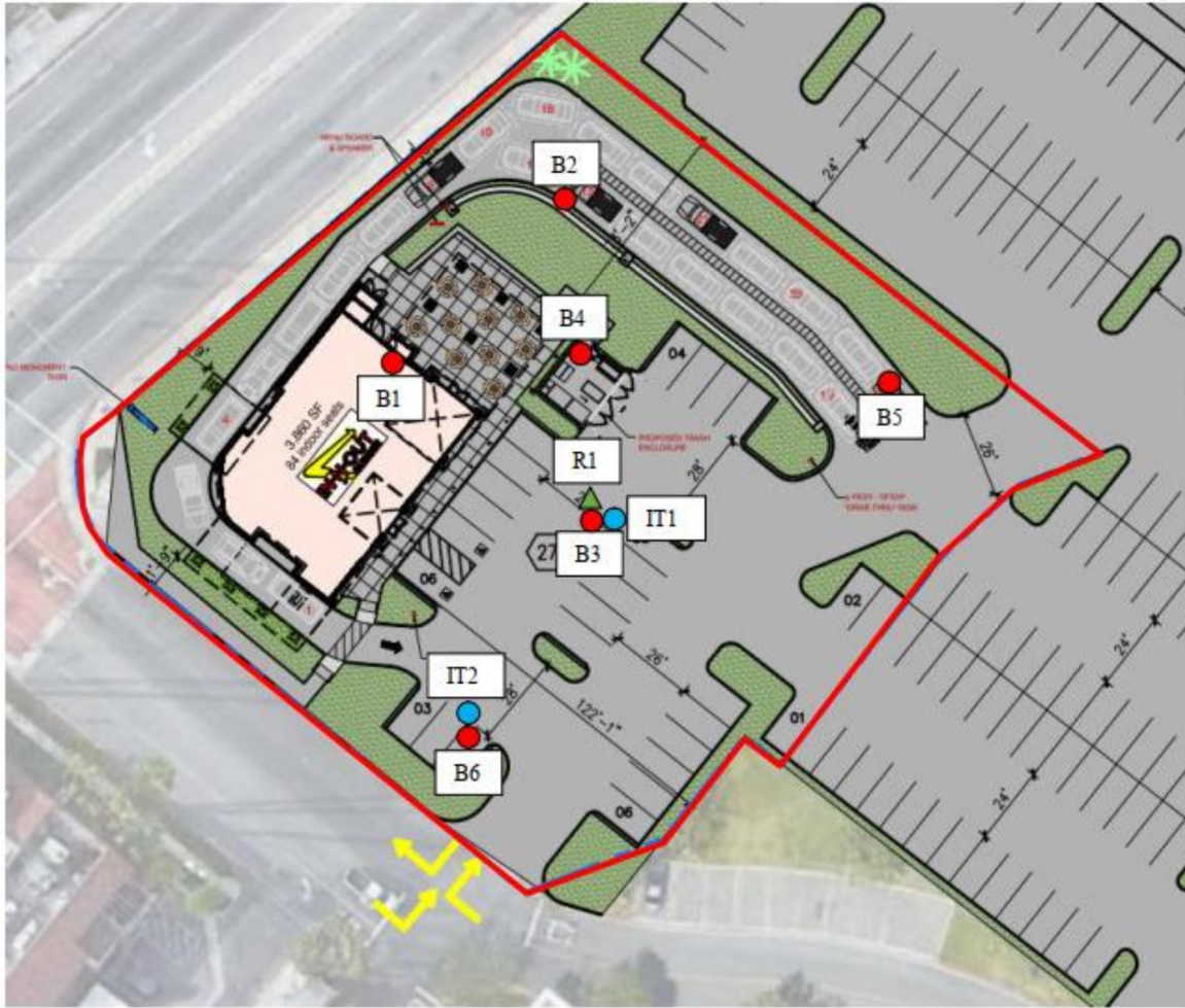
Figure 4 Subsurface Exploratory Investigation Locations
