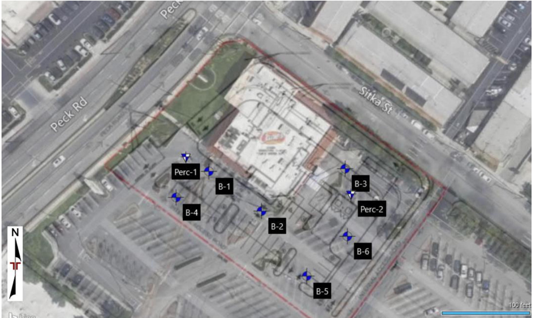
Figure 5 Subsurface Exploratory Investigation Locations
