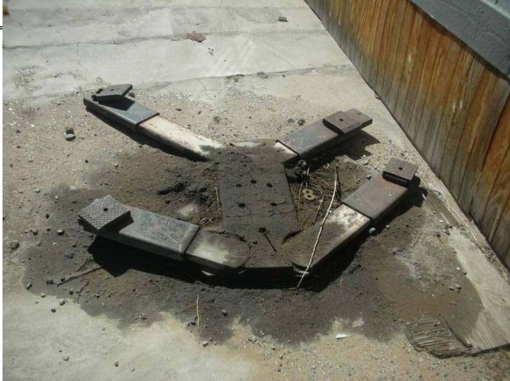
Photograph Number 7: Below-ground hydraulic lift next to the portable building in SW corner before removal
