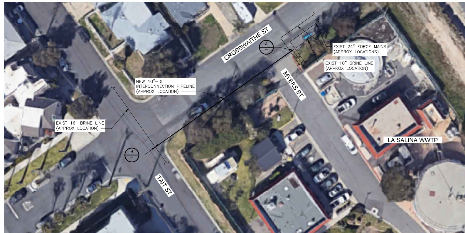
10" CONNECTION TO 16" AT LA SALINA WWTTP PLAN 1" = 20'
