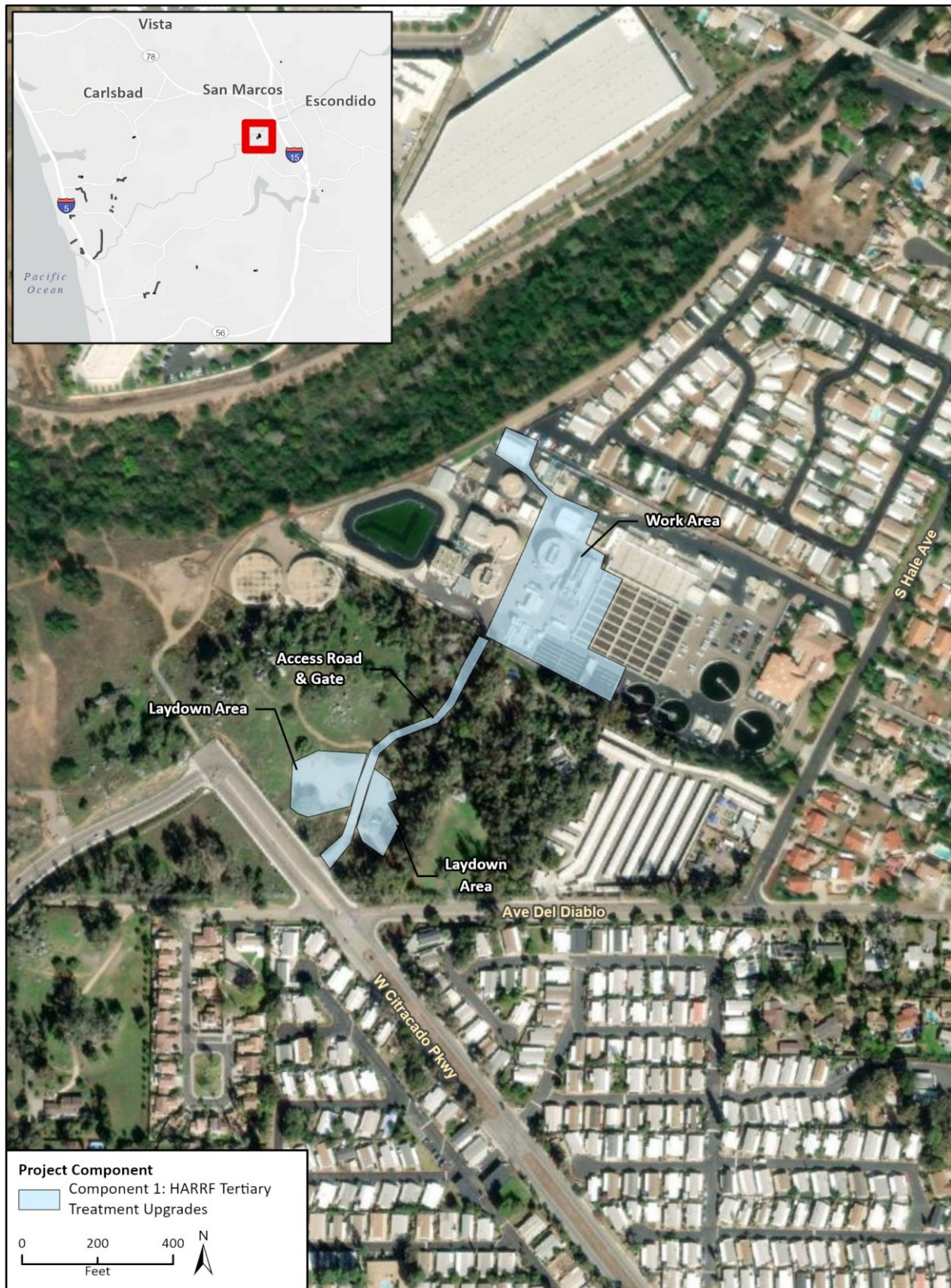
Figure 2 City of Escondido – Component 1 Location
