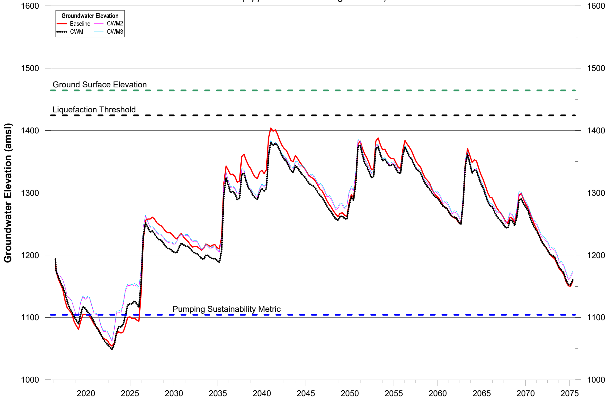
Figure 13a Model-Estimated Groundwater Levels for the Baseline Alternative and CWM-1,-2,-3 at Mountain View 4 Well (Upper Claremont Heights Basin)
