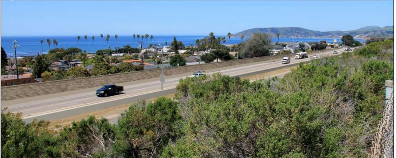
At this location, the project would add the part-time travel lane in the southbound direction and replace the existing concrete median barrier with a new, taller one. The 30-foot-tall lane control signals and camera poles would be seen in the median at between 7 and 10 locations along the freeway. If a soundwall were constructed at this location, this image shows how it could appear from this vantage point.
