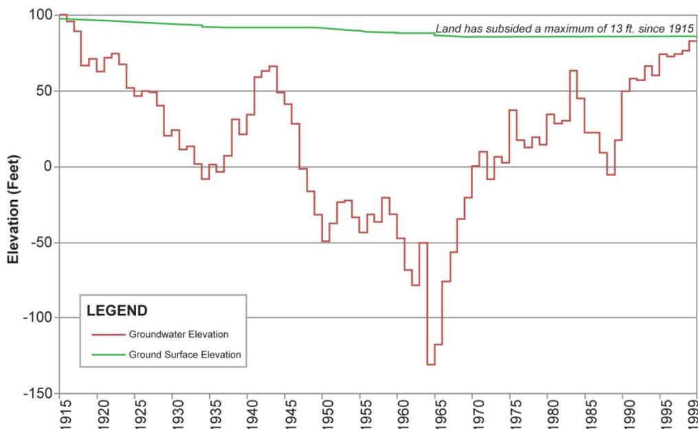
**Figure J-10. Land Subsidence at San Jose Index Well (Source SCVWD 2000)**
