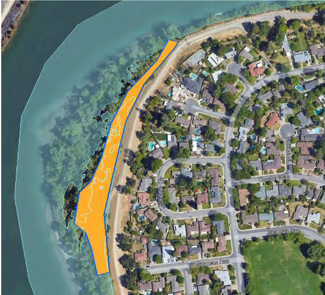
Figure 2. Overview of the staging area in the Little Pocket that is partially below the ordinary high-water mark. The staging area is the orange polygon and the ordinary high-water mark is shown by the light blue area.
