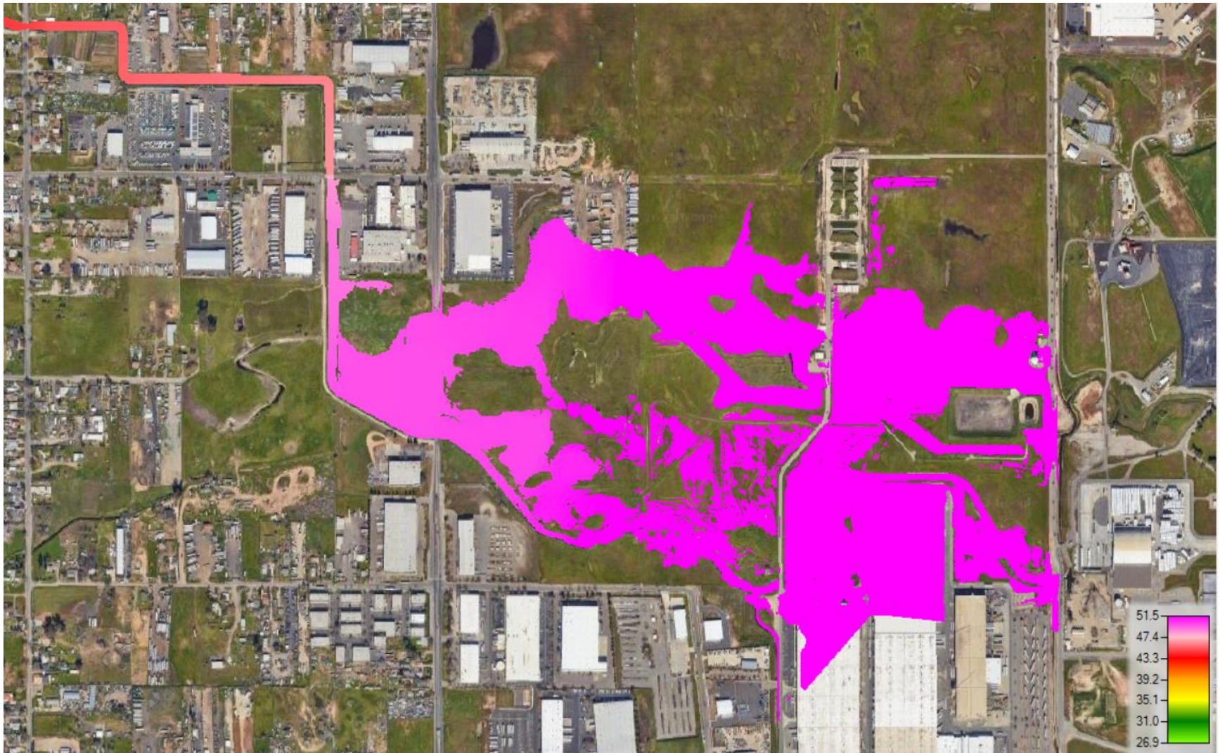
Figure 23: 10% (10 year) AEP Post-Project WSE – Intersection of Vinci & Raley
