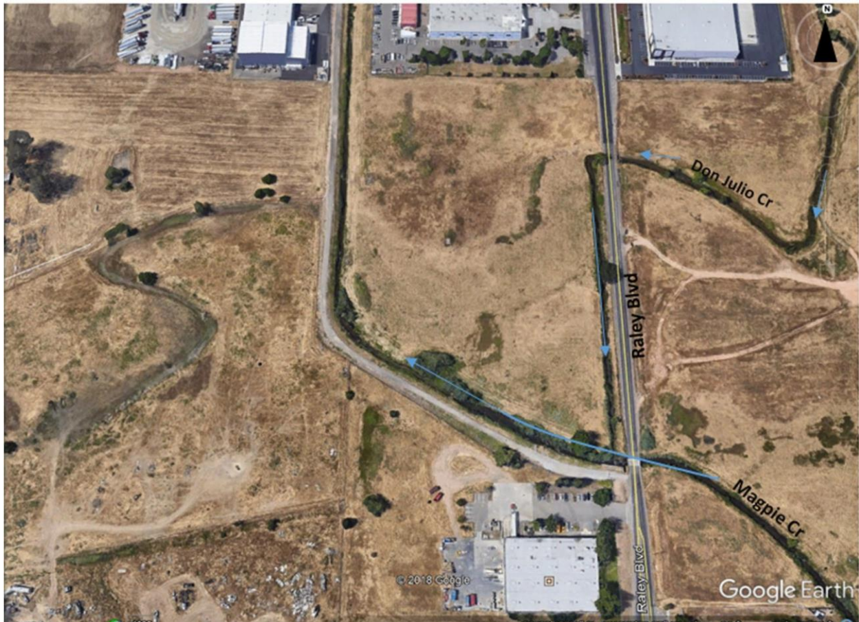
Figure 3-1 Magpie -Don Julio Cr Confluence and diversions. Don Julio Cr comes in from the upper right and is diverted below Raley BLVD to Magpie Cr which comes in from the Lower Right. Magpie Cr is then diverted northwest and north along the prominent levee to Robla Cr. The old Magpie and Don Julio Cr converge on the left side of the photo and are overflow channels for larger events.
