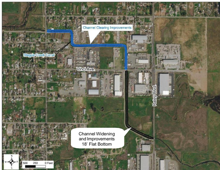
Figure 4-1: Channel Improvements Site Plan
