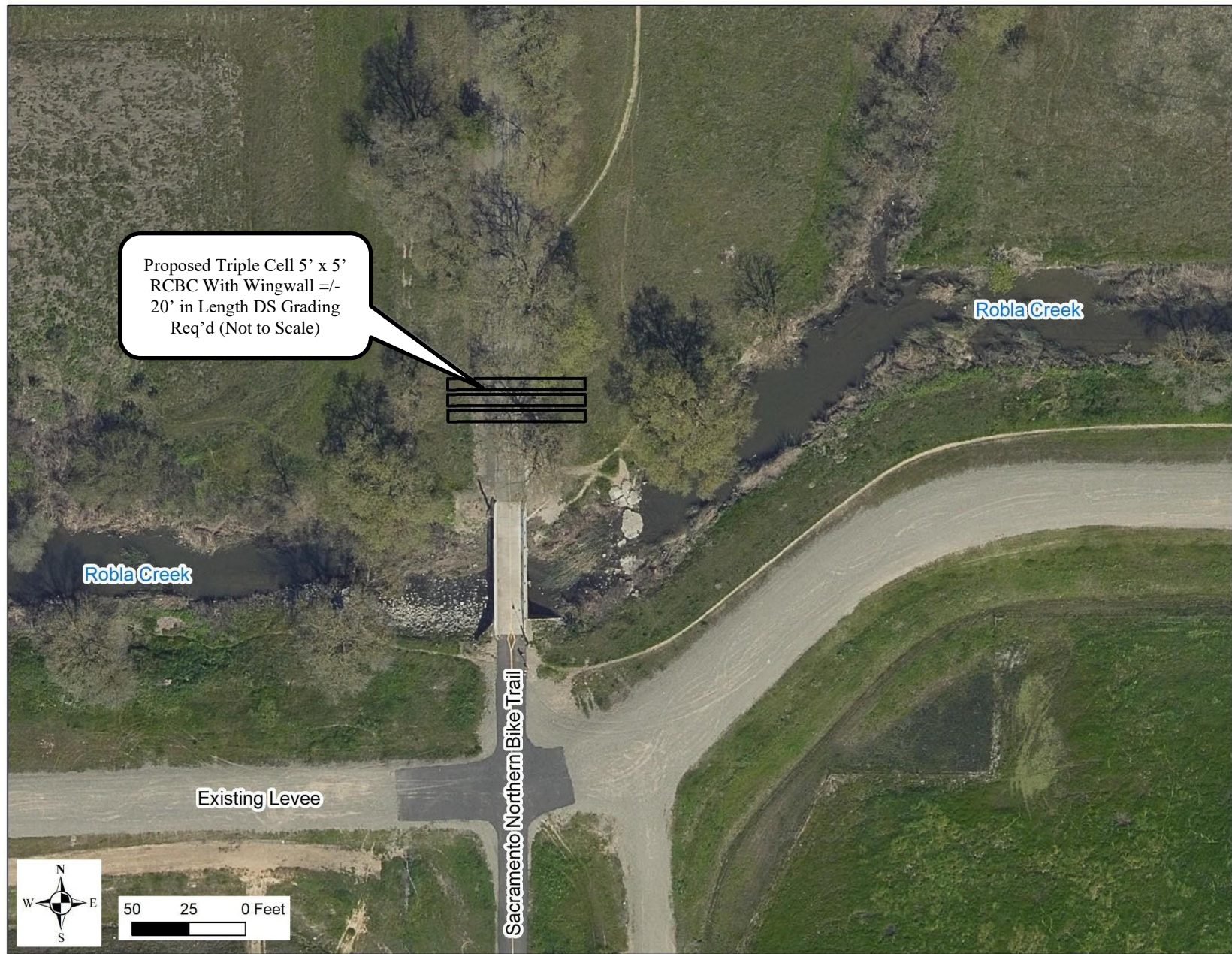
Figure 3. Aerial View of Culvert Design
