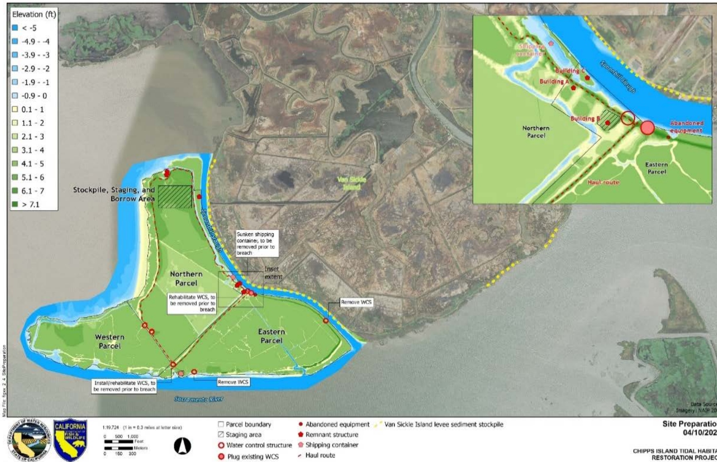
Figure 2-3. Site Preparation. The northern staging and stockpile area will encompass less than five acres and will be located within the larger area indicated on this map.
