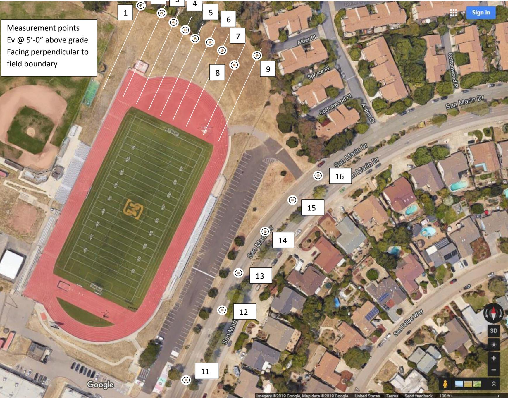
**TABLE A – VERTICAL PLANE MEASUREMENTS AT 5’ ABOVE ADJACENT GRADE ALONG AXIS TO FIELD CENTERLINE**
