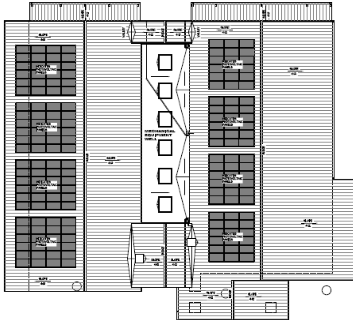
Figure 4.1-6 Roof Plan with Solar Panels
