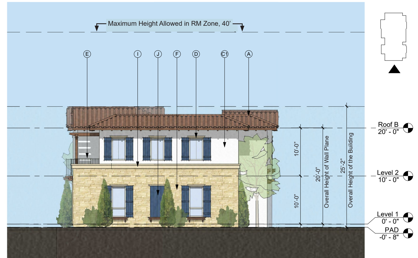
Building 8 - Elevation South
