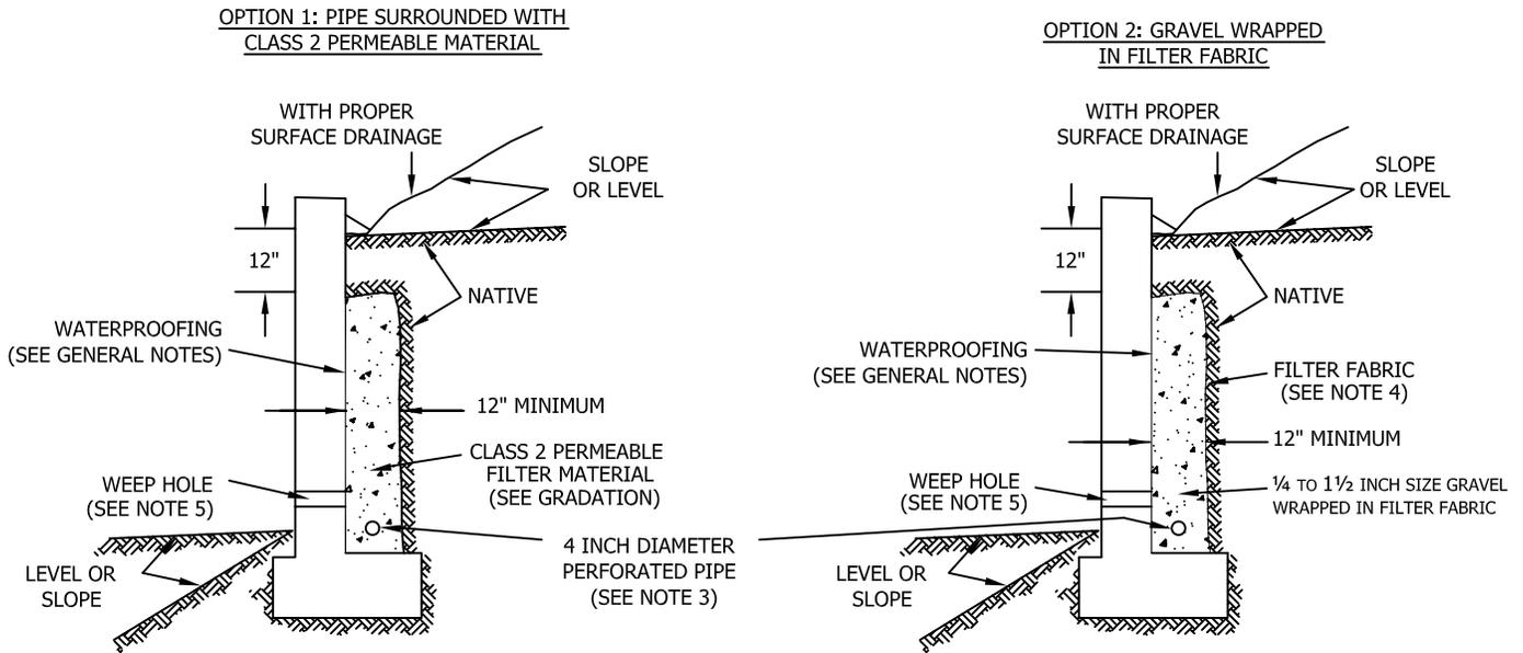
Class 2 Filter Permeable Material Gradation
