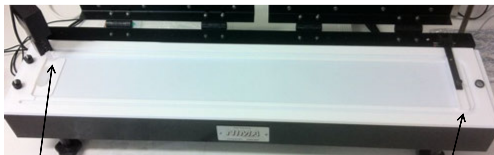
Surface pressure sensor (Wilhelmy plate)
