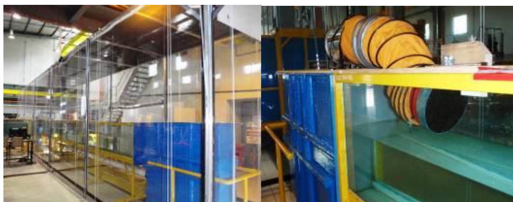
Figure 10: The wind and wave tank set-up showing the external structure enclosing the tank and the blower situated above the water surface. (Photograph: P. Schouten).
