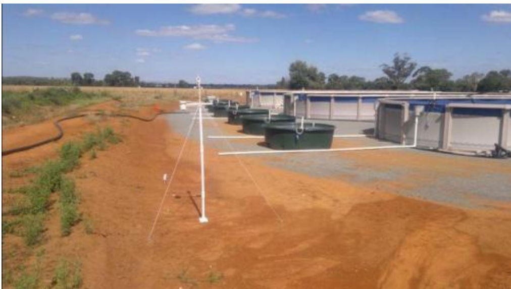
Figure 17: New layout of the six troughs for Trial 3 onwards (shown alongside the three large evaporation ponds). (Photograph: A. Leung)
