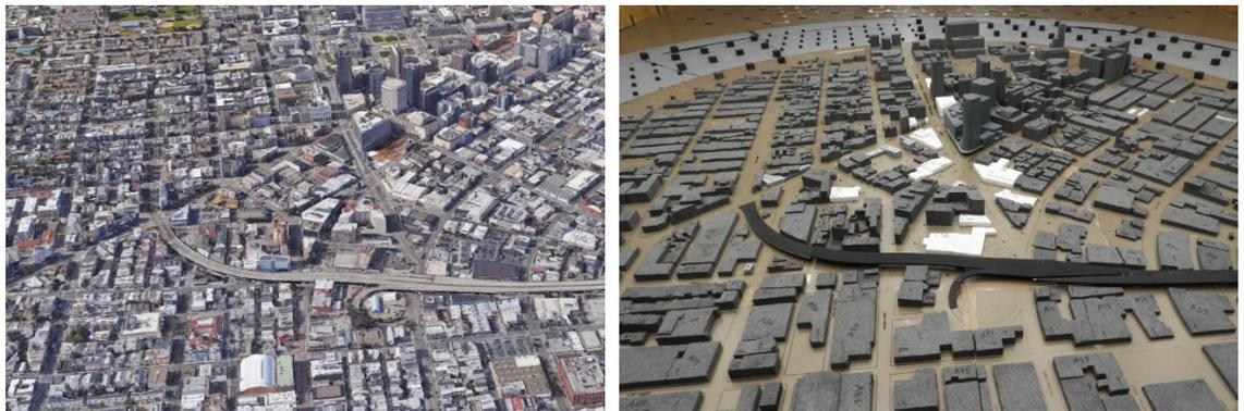
**Google Earth Photo (left) and Wind Tunnel Model (right) for the Hub Area**
