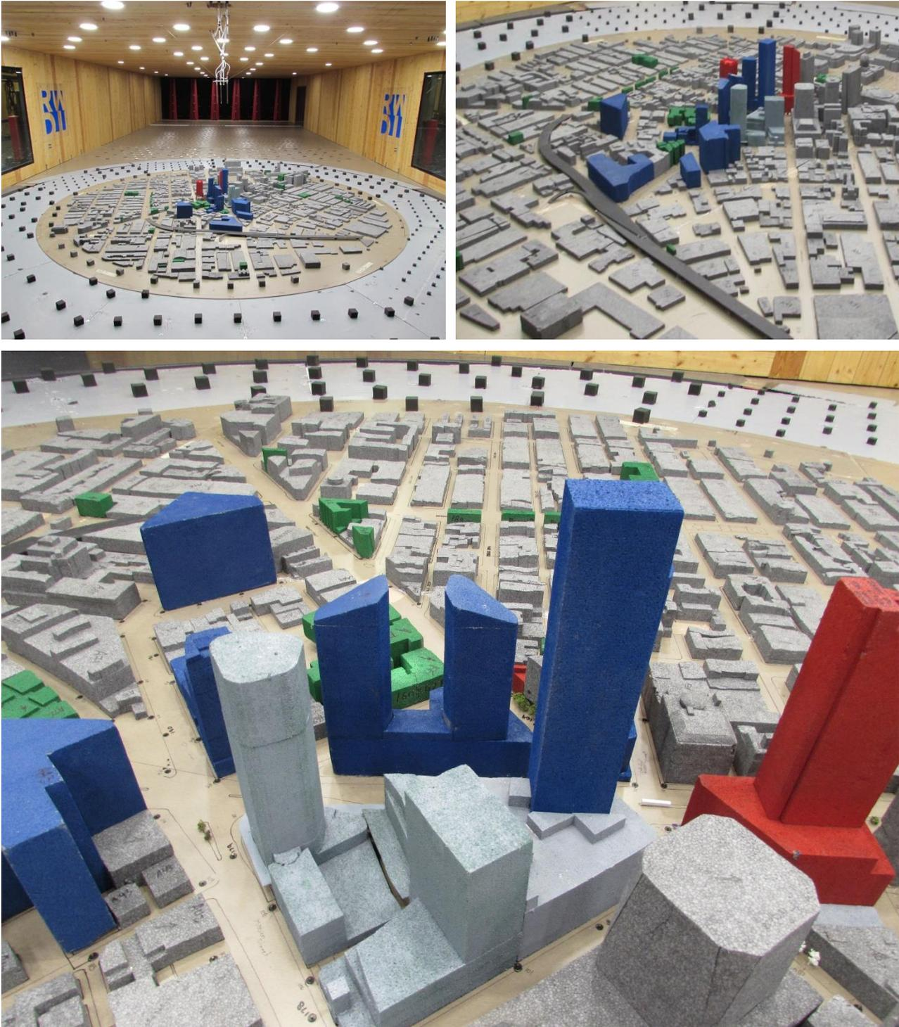
Image 2d: Wind tunnel study model – Cumulative 2 configuration
