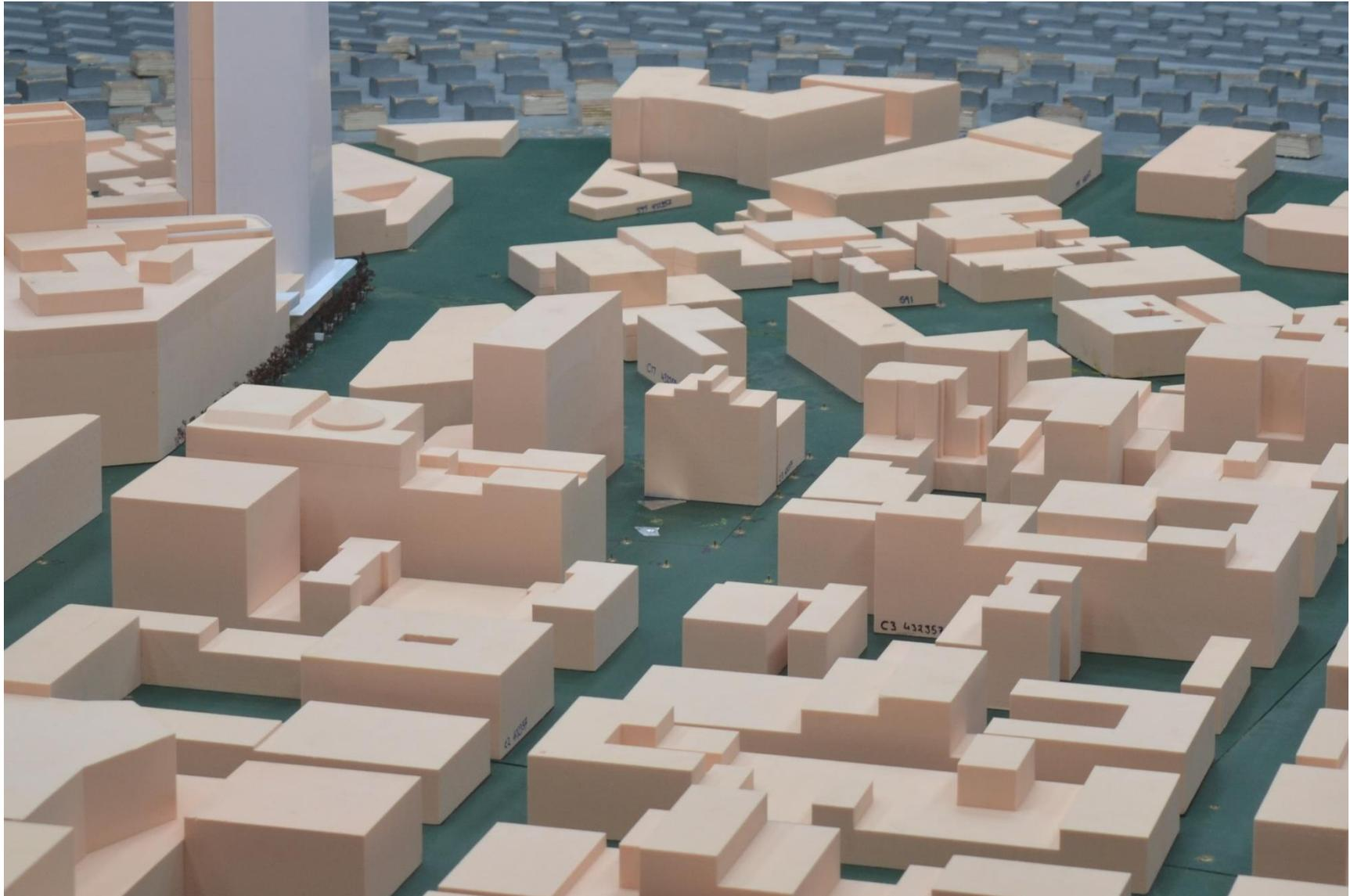
Figure D.2: Existing Scenario, Wind Tunnel Setup, Viewed from Southeast
