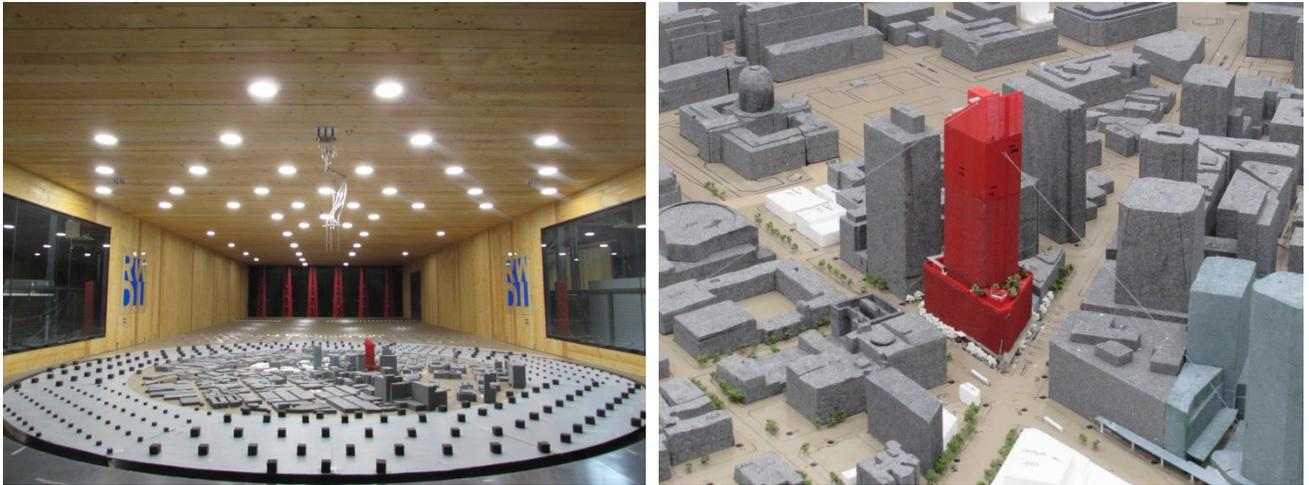
**Image 2b: Wind tunnel study model – Existing + Proposed configuration**
