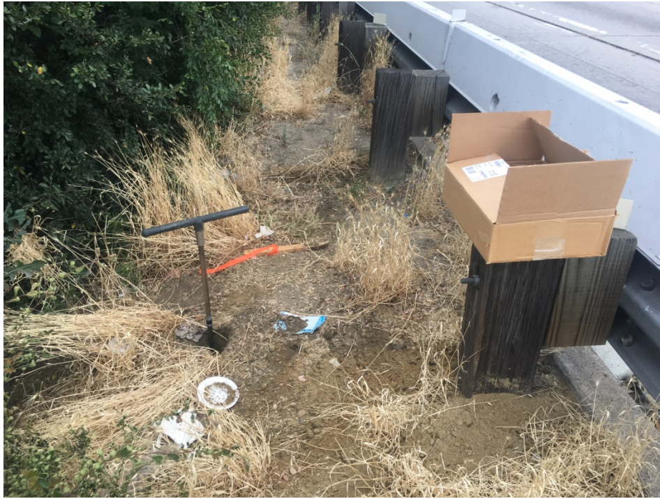
a. Hand Auger Sampling at ADL Boring in Area 9
