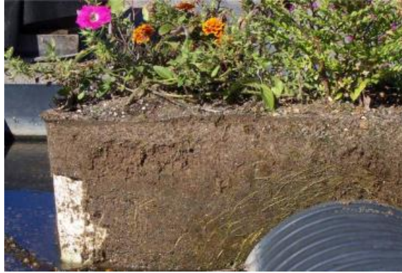
Figure V - EPIC sand capillary zone above saturated zone
