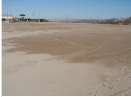
Figure- Capillary rise witnessed at surface as level EPIC field is charged from inlet header to outlet header.
