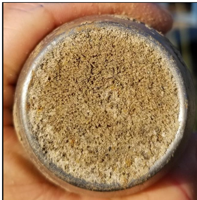
Figure 4-3. Very Old Paralic Deposits in Boring B-1
