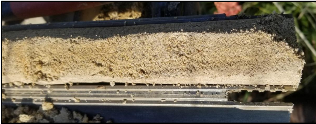
Figure 4-4. Scripps Formation in Boring B-2
