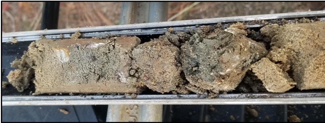
Figure 4-2. Fill at Boring B-1
