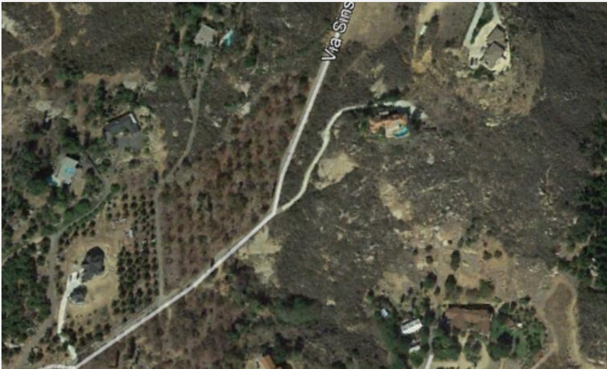
Figure 8. Example of “lower density” development where structures are interspersed amongst wildland fuels, are of varying ages, and include varying levels of fuel modification zone setbacks. Homes are exposed on most or all sides by flammable vegetation and properties rely solely on owners for maintenance, are often far distances from the nearest fire station, and have minimal buffer from on-site fire spreading to wildlands.
