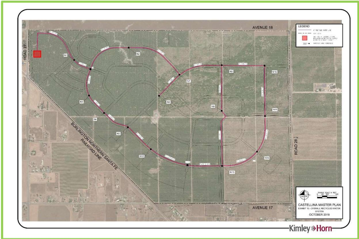
Figure 2 – Overall Recycled Water System Layout
