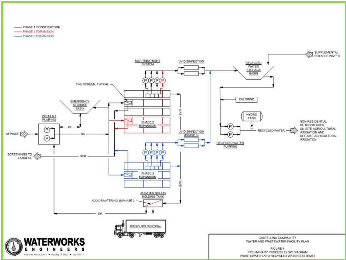
Exhibit 14 - Wastewater Treatment System Schematic
