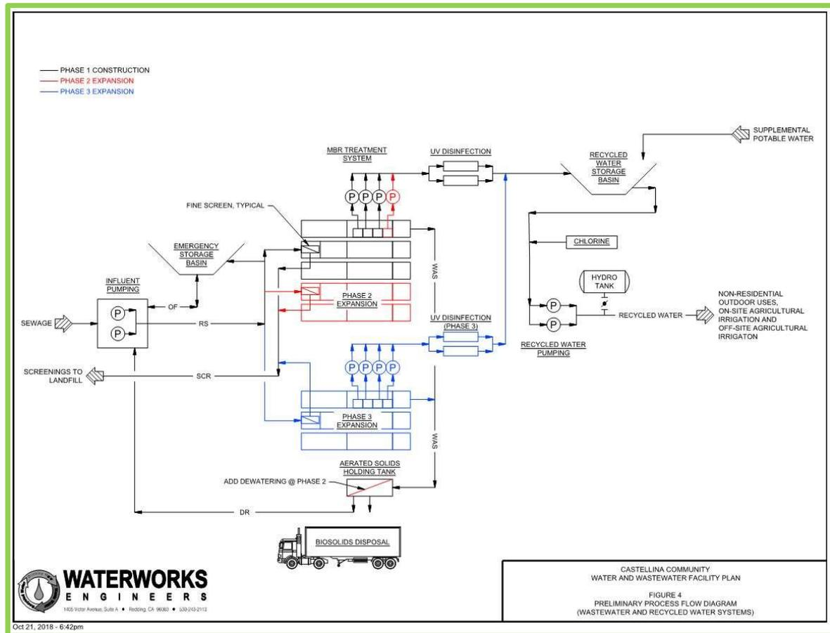
Figure 5 – Wastewater and Recycled Water Facility Process Flow Diagram
