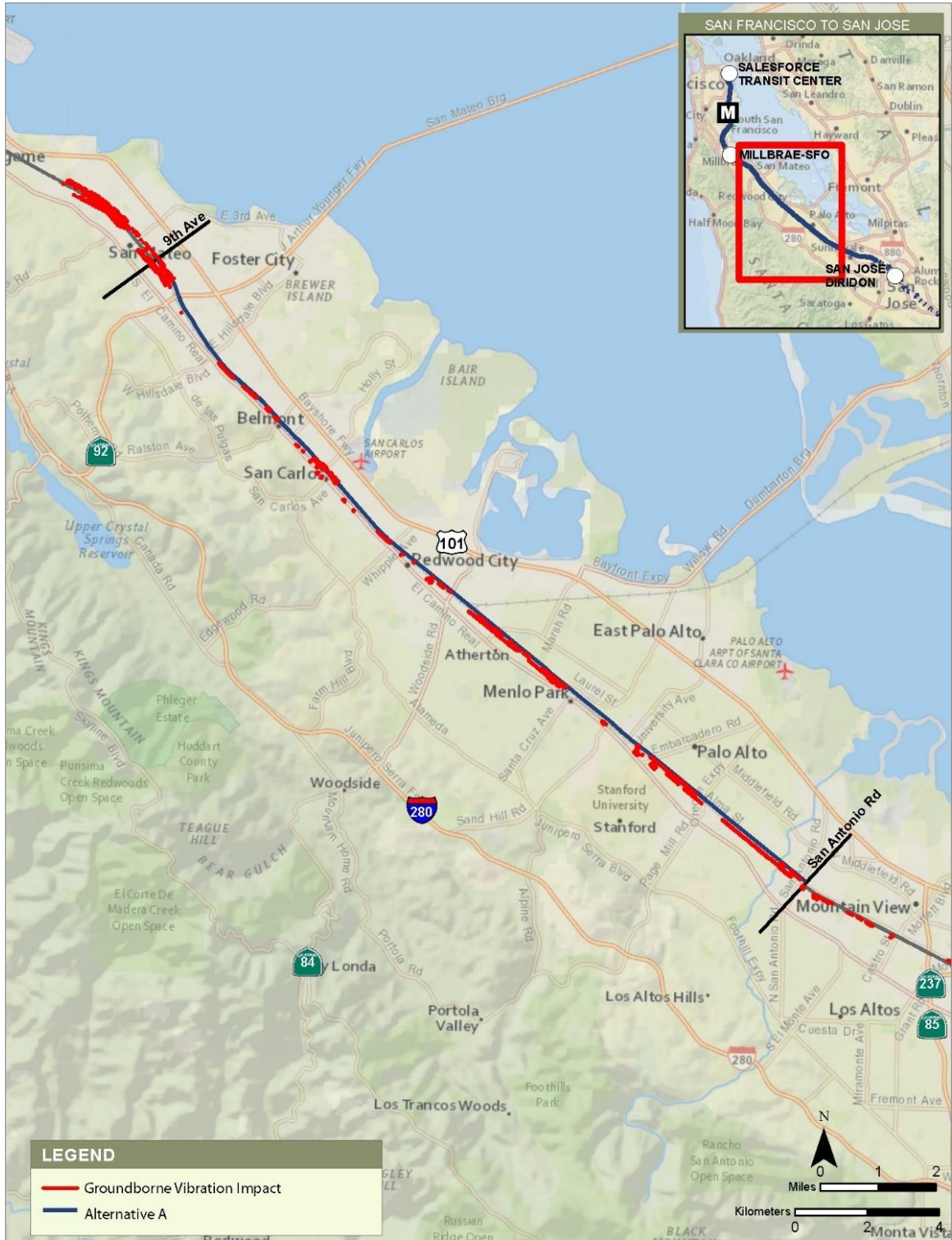
Figure 5-18 2040 Plus Project Vibration Impacts—Alternative A (San Mateo to Palo Alto Subsection)
