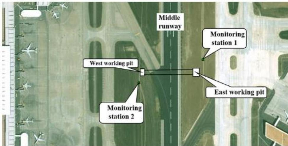
Figure 4-5: Monitoring Stations Used during Construction for Monitoring Ground Movements
