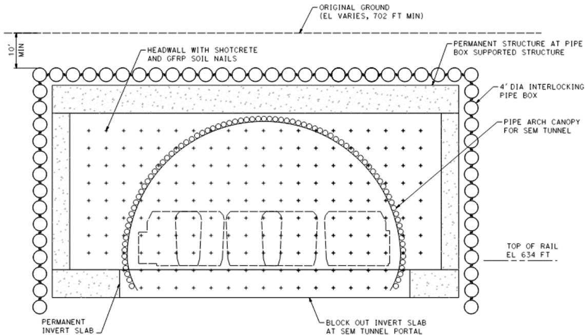
**Figure 1. Typical Cross Section of Box Tunnel Excavation with Interlocking Pipes**
