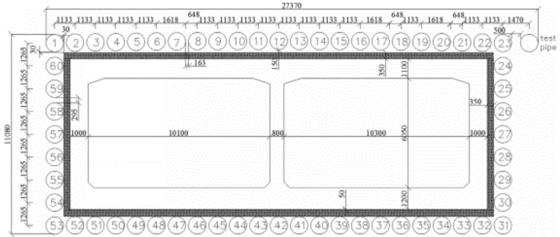
Figure 4-4: Finished Cross Section of the Twin Tunnels and Pipe Layout
