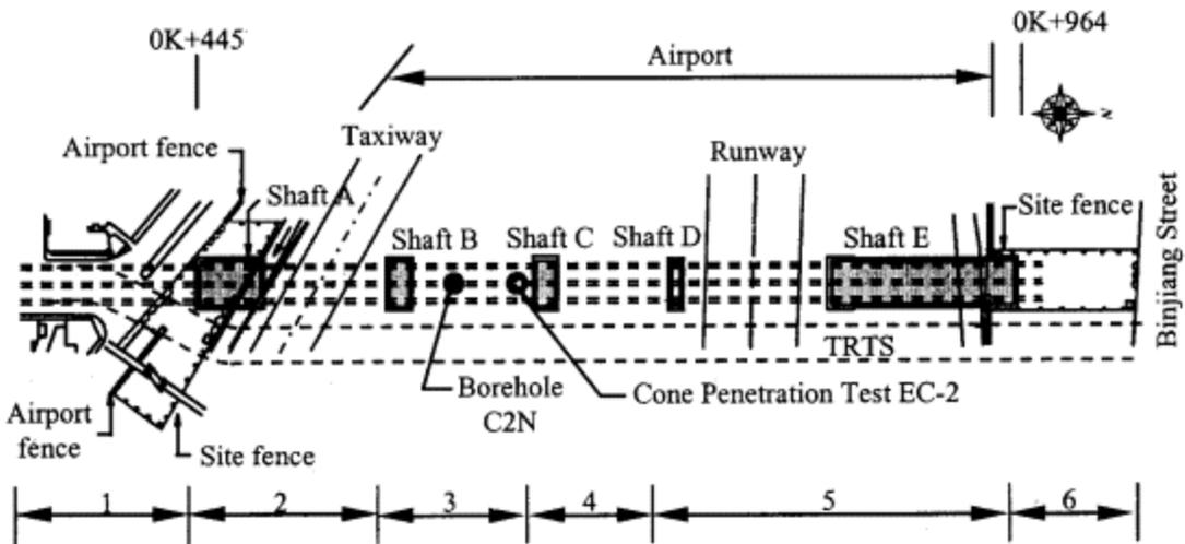
Figure 3-2: Construction Site Plan
