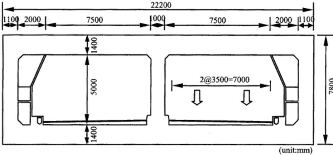
Figure 3-5: Finished Tunnel Cross-section
