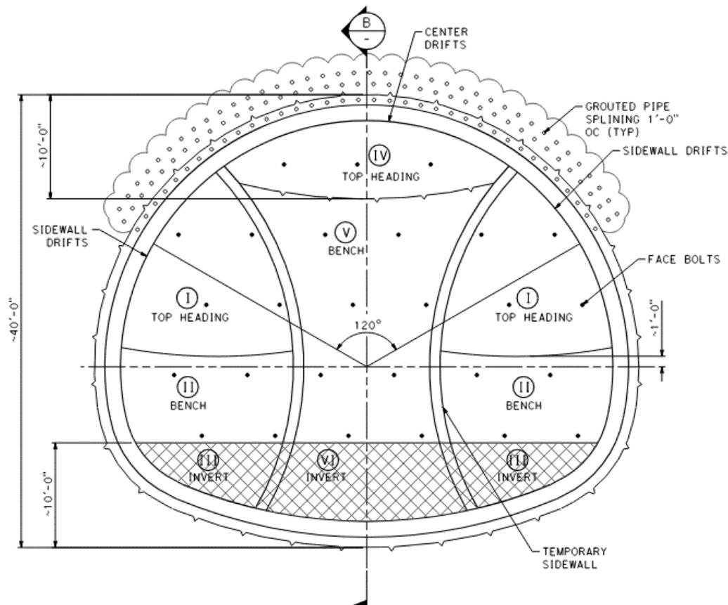
**Figure 2. Sequential Excavation Method Construction Sequence**
