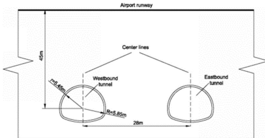
Figure 6-2: Section View of Tunneling Under Runway
