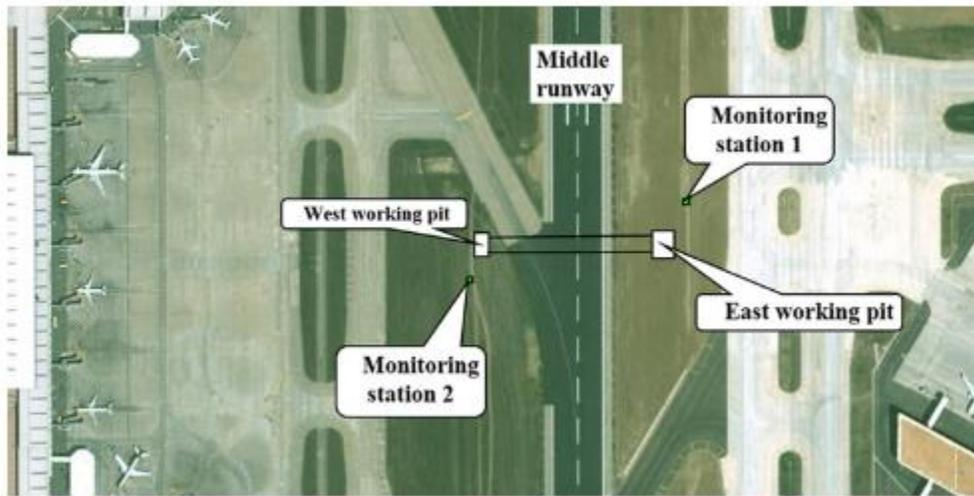
Figure 4-5: Monitoring Stations Used during Construction for Monitoring Ground Movements
