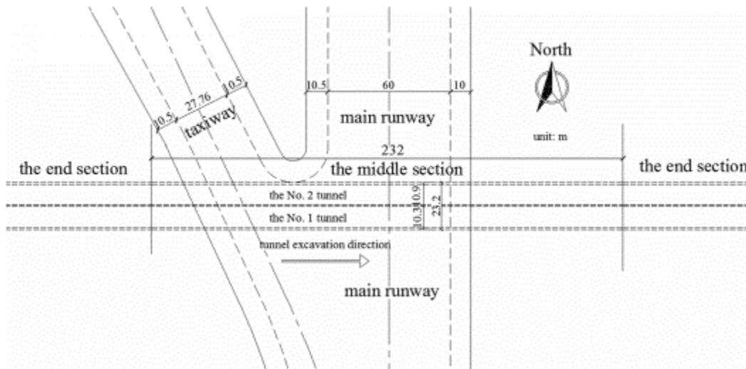
Figure 4-2: Enlarged Plan of the Tunnel and Runway Sections
