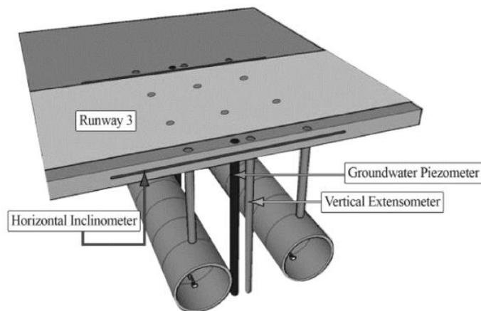
Figure 5-3: Geotechnical Monitoring and Tunneling beneath the Runway
