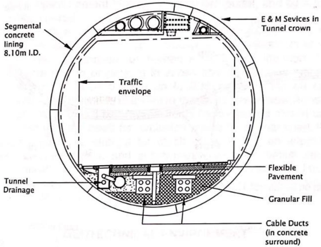
Figure 1-3: Tunnel Cross Section
