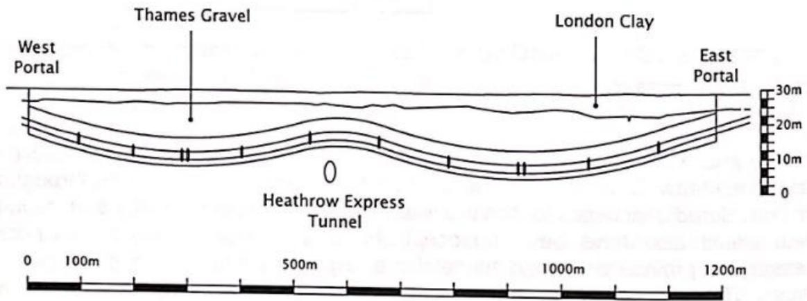
Figure 1-2: Tunnel Longitudinal Section
