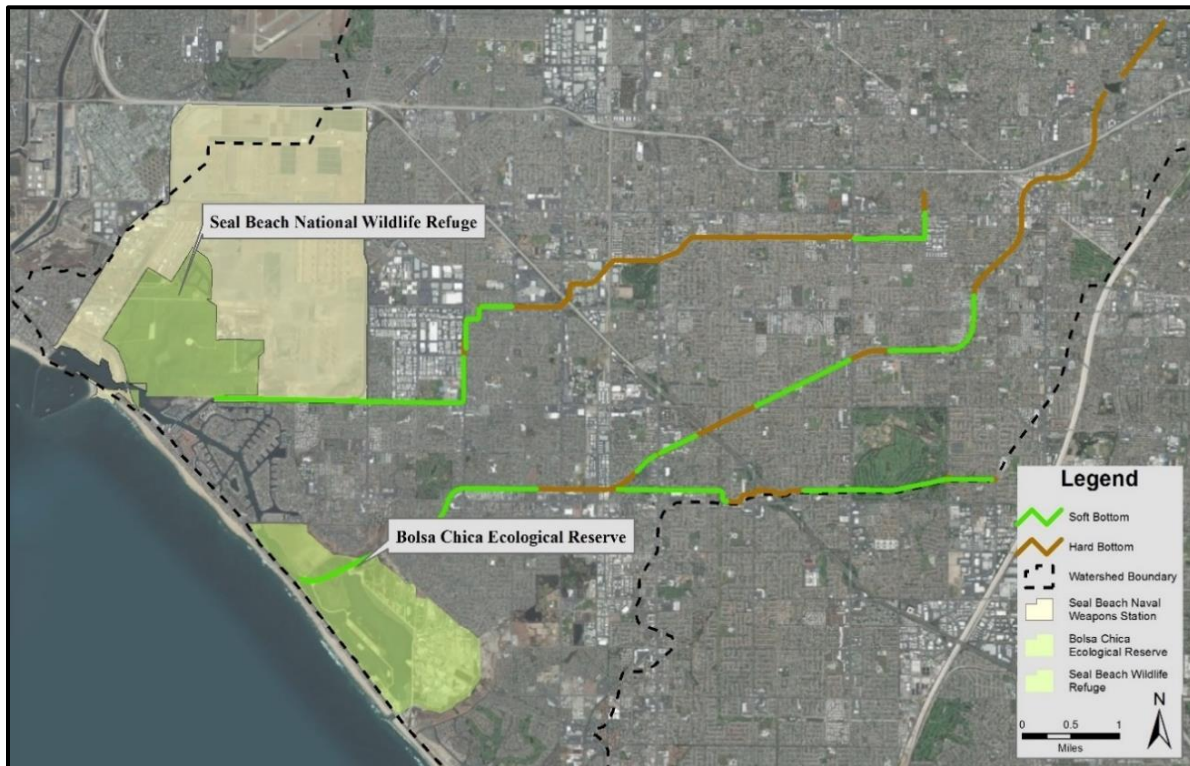
Figure 12: Existing channel bottom conditions.
