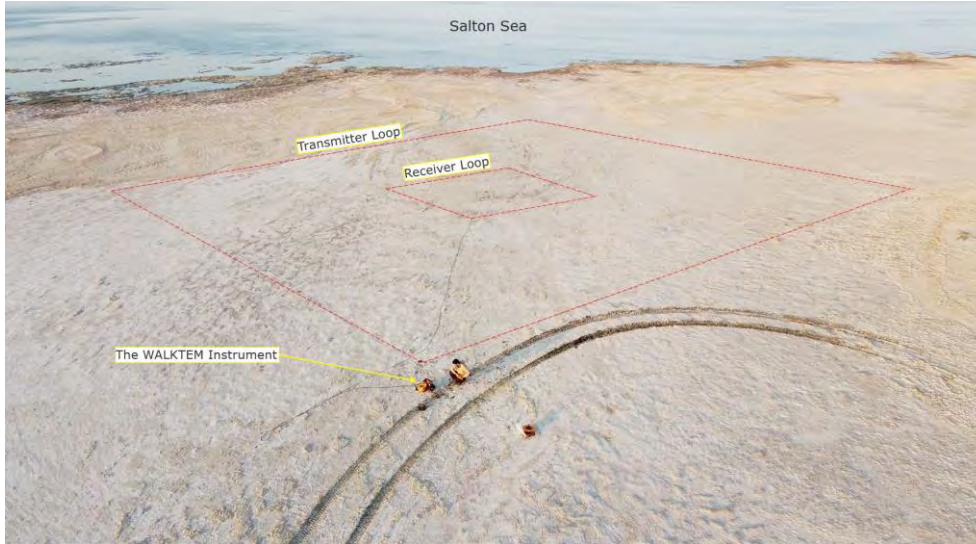
Figure 4 The WalkTEM instrument in operation at the Bombay Beach.
