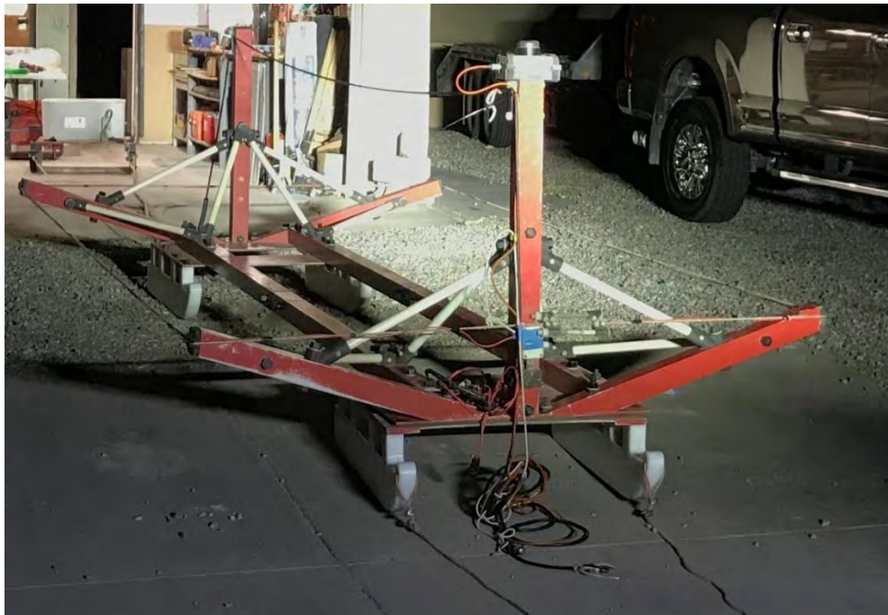
Figure 3 The tTEM transmitter sled setup at the Formation field house.
