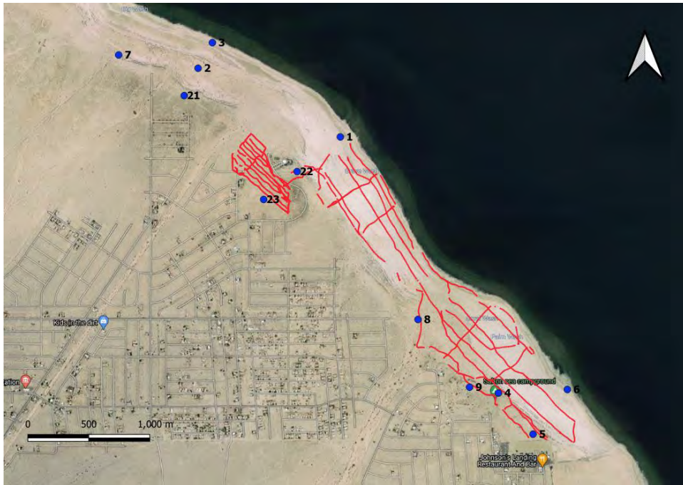
Figure 6 Location map of the tTEM survey lines and WalkTEM soundings at the Clubhouse. tTEM survey lines are marked as red dots and WalkTEM sounding locations are shown with blue circles.
