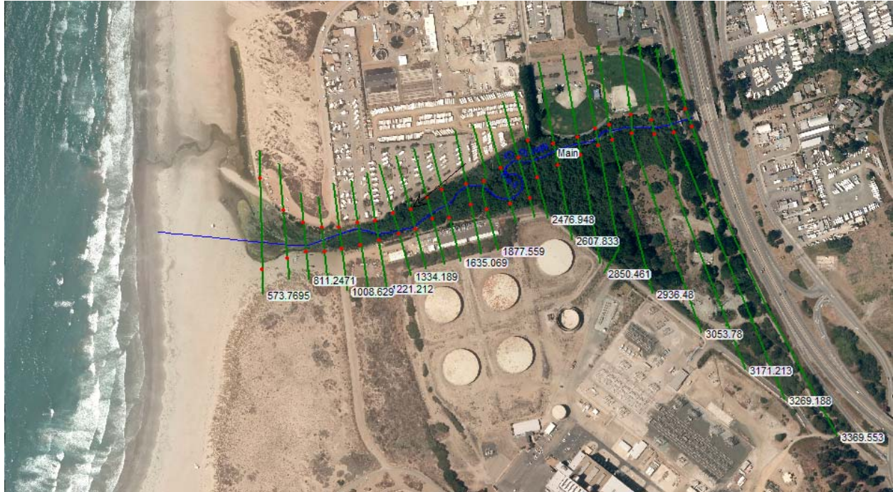
FIGURE 13: HEC-RAS MODEL LAYOUT FOR MORRO CREEK
