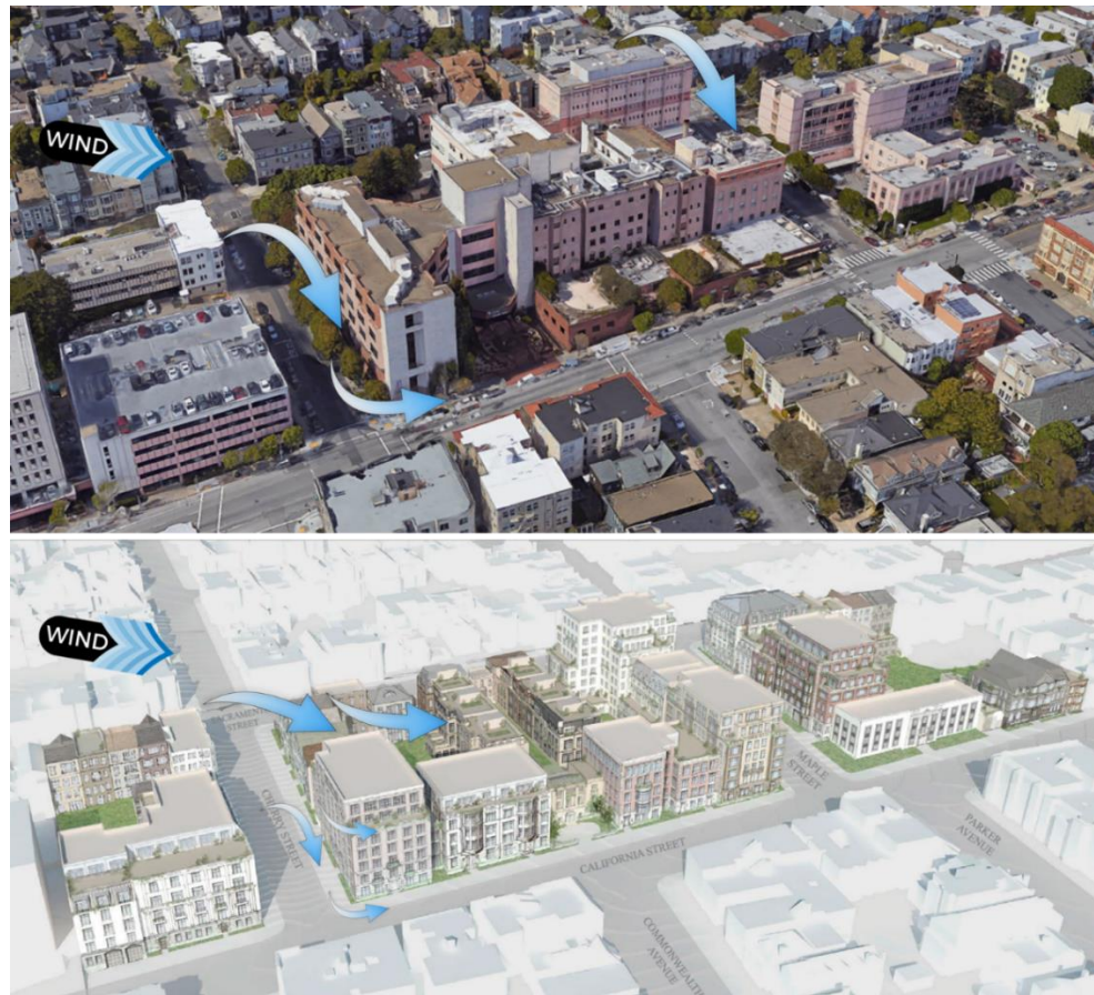
Image 6: Anticipated Wind Flows through the Existing (Top) and Proposed (Bottom) Development
