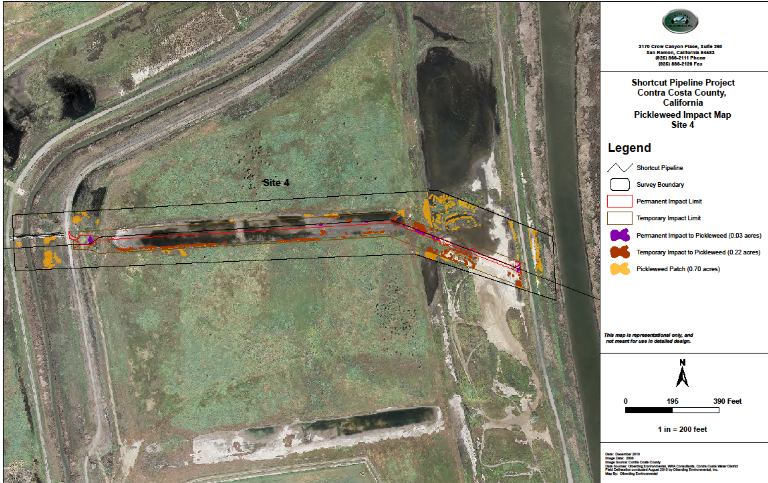
Figure 17 - Permanent and Temporary Impacts for Pickleweed at Site 4
