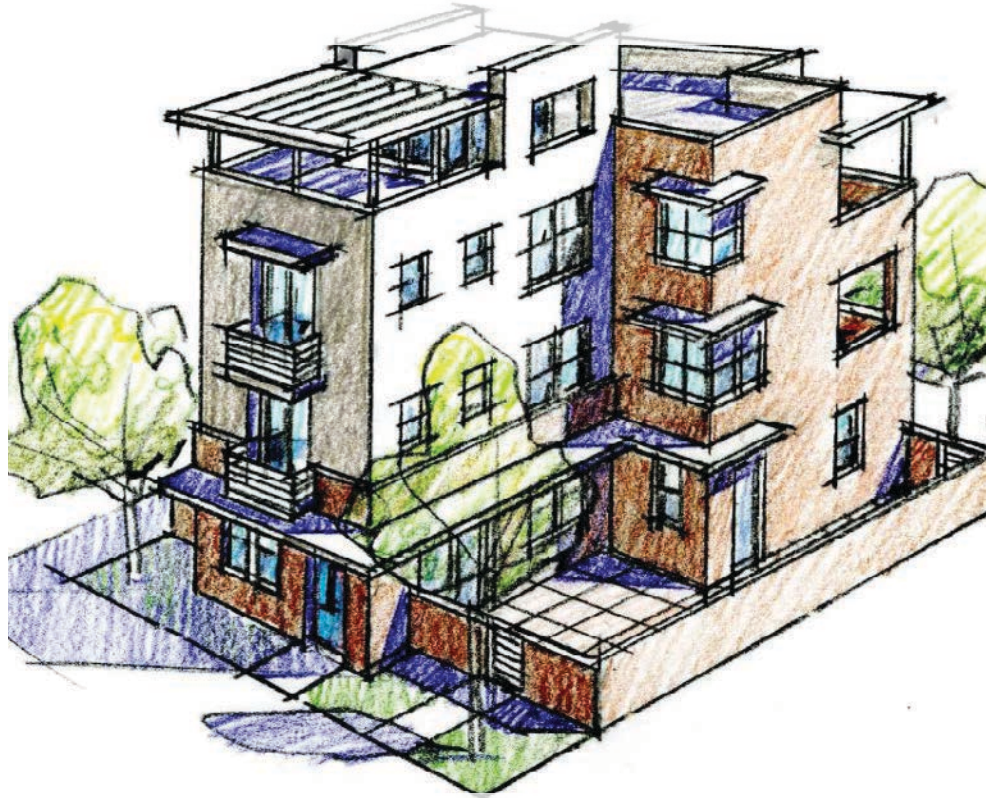
Portions of wall extend above the body of the building to emphasize areas and create interest
